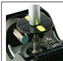
Fig. 5: Removing indicator
